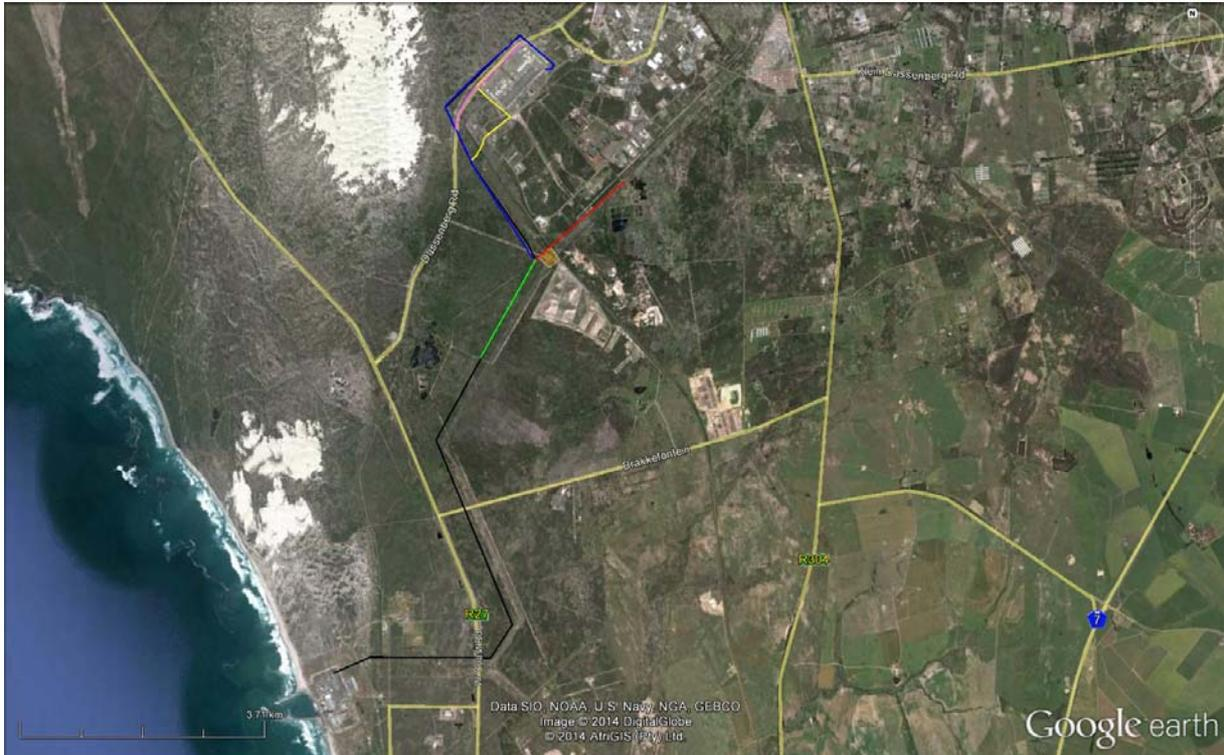
**Figure 1.** The proposed changes to the Koeberg-Ankerlig line, illustrating the various sections of the line as follows: the decoupling will occur somewhere along the green section of the line, the red section would no longer be required and would be decommissioned and the blue section illustrates the approximate route of the new alignment Alternative 1, with Alternative 2 in pink, Alternative 3 in yellow and Alternative 4, outlined in orange.
